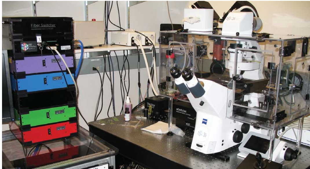
One of the new additions to the Integrated Microscopy Core Facility, the Marianas Nipkow system is a high-powered light microscope that allows researchers to study living cells.
